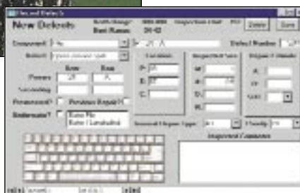
The inspector inputs data for each specific defect, allowing systematic development of an estimate using the AIRIS program.
