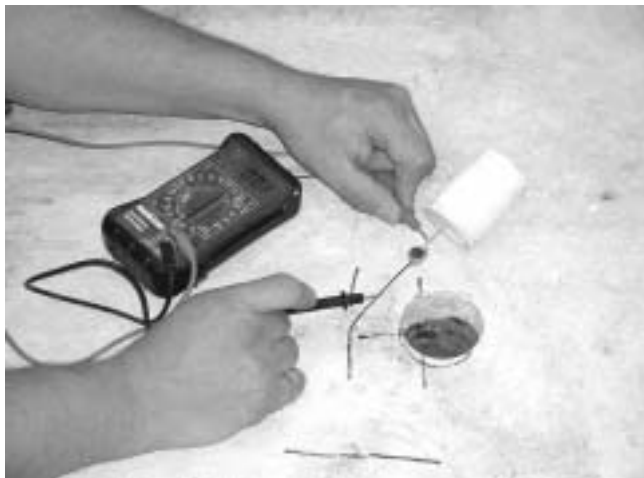
Fig. 12—Confirming connection to reinforcing steel.
