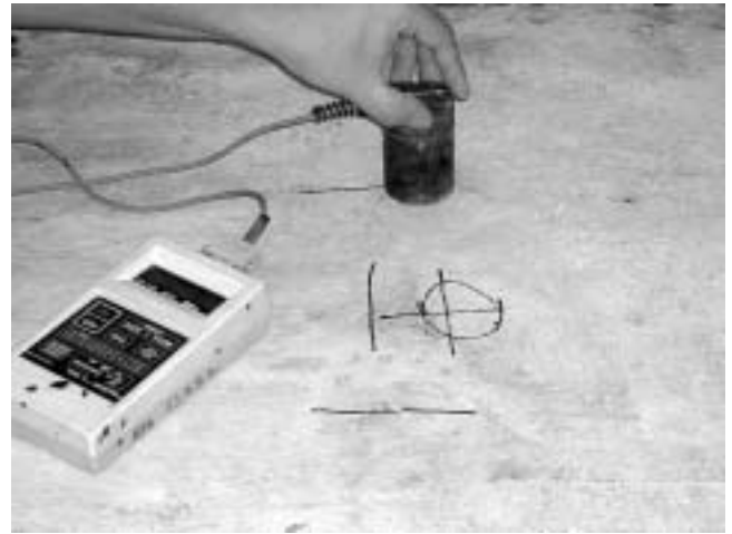
Fig. 9—Locating reinforcing steel.
