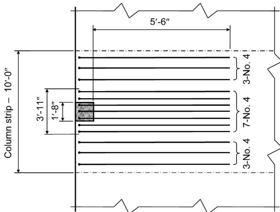
Check the combined shear stress at the inside face of the critical transfer section.
