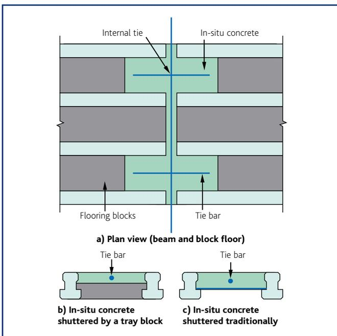
The tying requirements for Class 2B buildings or above can be achieved by placing horizontal ties within the depth of the floor. Figures 13 and 14 show typical details for hollowcore (also see Section titled Precast framed structures) and beam and block floors.
