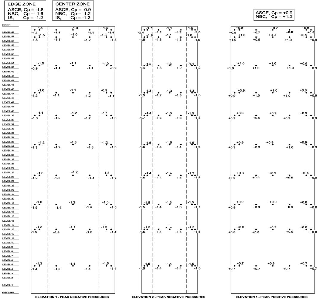
Figure 4. Peak pressure coefficients on CAARC facades.
