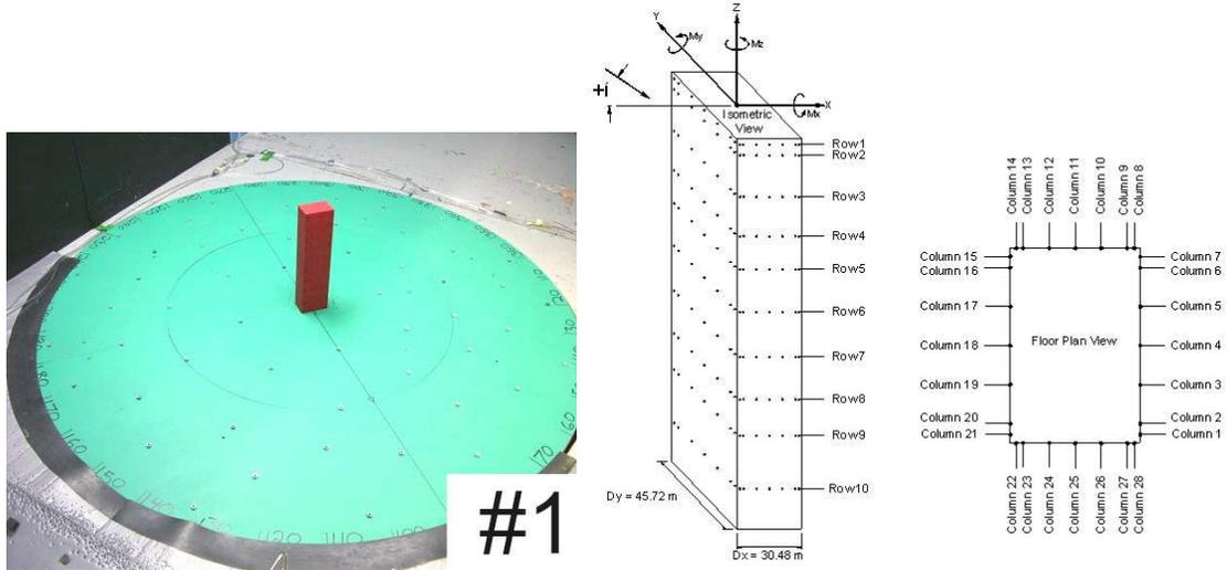
Figure 1. CAARC building model in wind tunnel - pressure tap locations.
