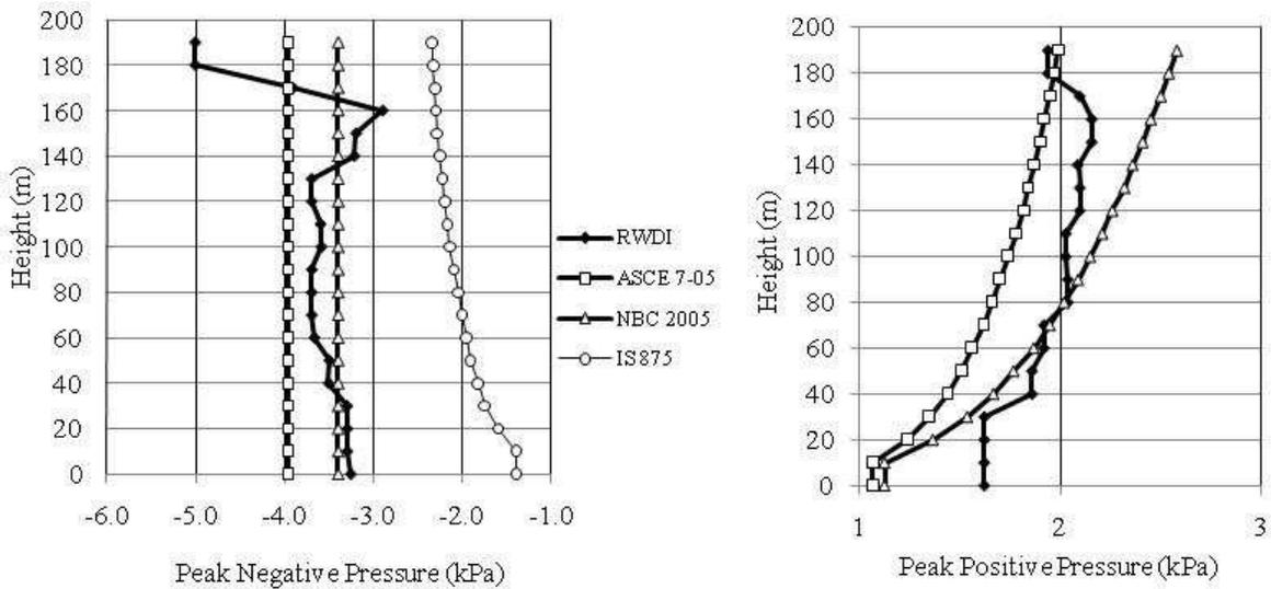
Figure 5. Comparison of peak pressures on CAARC building.
