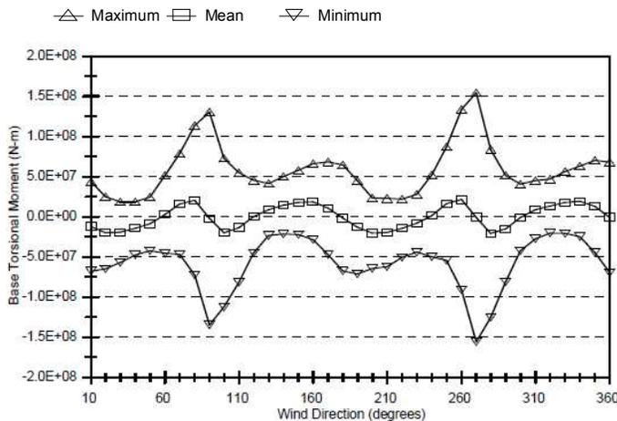
Figure 8. Overall torsional moment on CAARC building.
