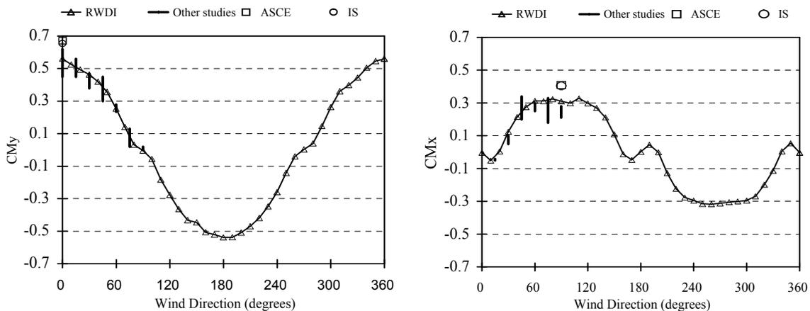
Figure 6. Wind-induced mean response of CAARC building.
