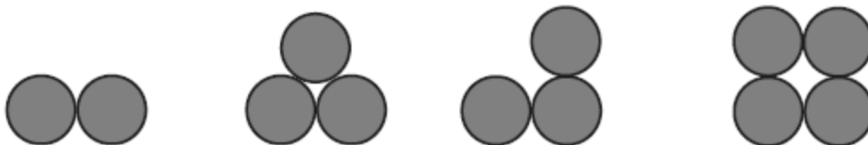
Figure 3-2 Possible Reinforcing Bar Bundling Schemes
